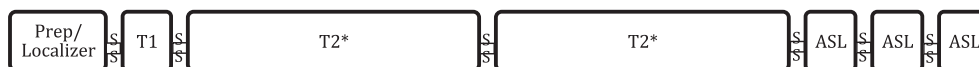
Fig. 1. Image-data acquisition time line. Prep = subject preparation, including placement of sound-attenuating ear plugs, adhesive electrodes, and foam head restraints. Localizer = anatomical localization scan to position the imaging volume. T1 = T1-weighted anatomical scan. T2* = 15 min BOLD image-volume acquisition for ICN analysis. ASL = 2.5 min arterial spin labeled acquisition. The number of epochs of T2* (1–3) and ASL data (3–5) varied across subjects, depending on sleep duration. SS = sleep-stage determination, which was performed between all imaging epochs.
